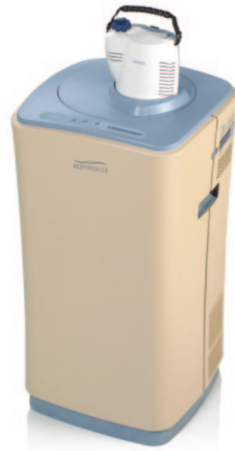
Fig. 6. HomeLOX liquid oxygen system, which creates oxygen from a concentrator and refrigerates the concentrator gas to a liquid state, which is stored in a small dewar to trans-fill to a liquid-oxygen portable. (Courtesy of Philips Respironics.)
