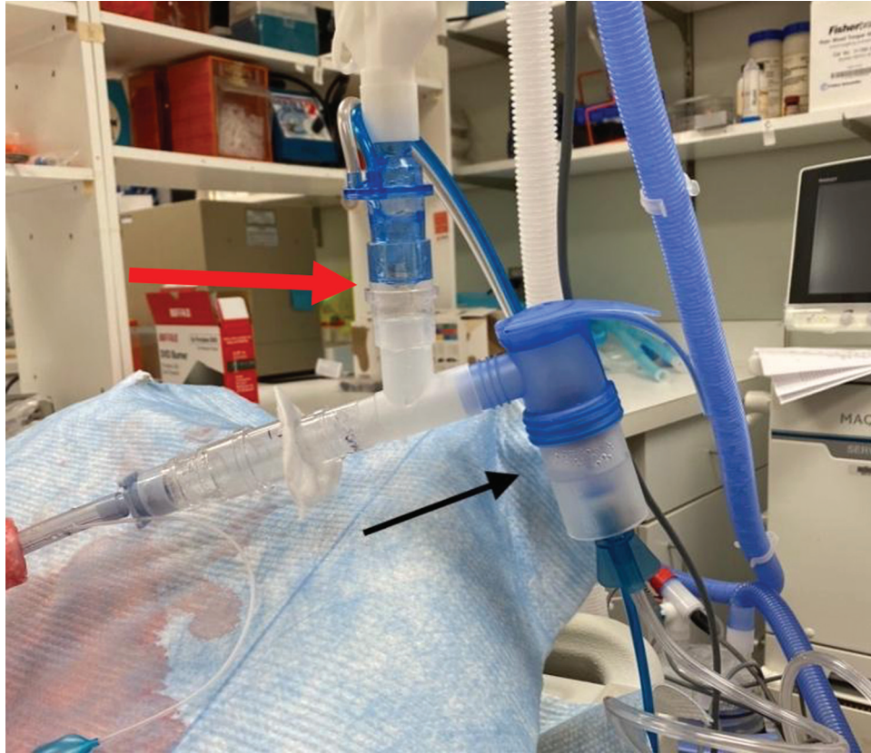
Fig. 3. The bottom black arrow indicates the location of the nebulizer in the ventilator circuit during Phase 2 of the experiment. The top red arrow in this image is the location of the viral filter to collect the simulated breath from the model.
