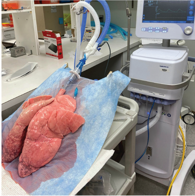
Fig. 2. Physical setup of the porcine model. The lungs are placed on a ramp to situate the lungs 30° relative to the bench surface. The connection between the ventilator circuit and the endotracheal tube is shown with the viral filter proximal to the endotracheal tube and distal to the Y-piece of the circuit connection. The background demonstrates the location of the mechanical ventilator used for the series of experiments.
